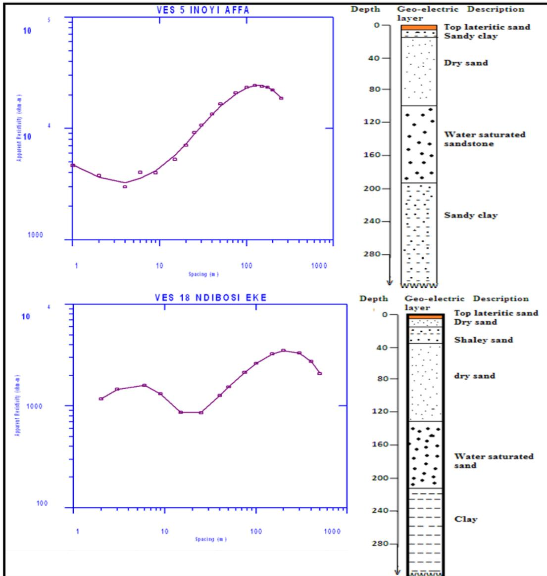
Fig. 5: Sounding curve and descriptive section for VES 5
